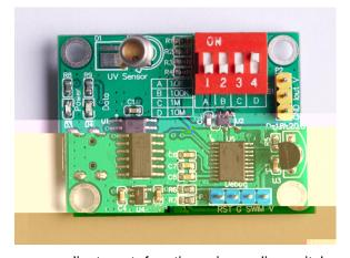
The evaluation board supports measurement range adjustment function via a dip switch.
