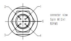
5-pin analog plug: pin  $1=V_{cc}$ , pin 2=null, pin  $3=I_{out}/V_{out}$ , pin 4=GND/null, pin 5=null
